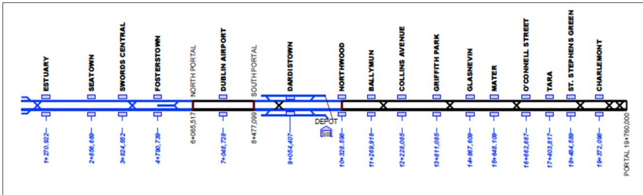
Figure 3-3: MetroLink Route with Track Crossings
